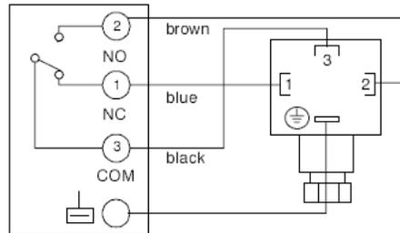
Fig.3. C6097A connection diagram with DIN plug
