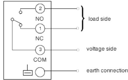
Fig.2. C6097A connection diagram
