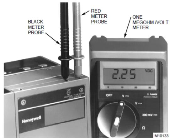
**Fig.10 Measuring voltage flame signal with 7800 Series control**
