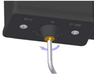
Figure 24: CPI switch adjustment
