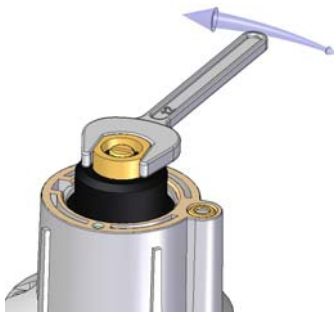
Figure 24: Adjusting flow rate.
