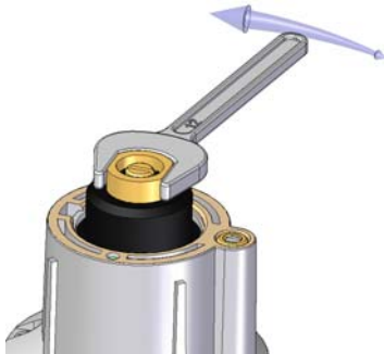
Figure 7 Adjusting flow rate.
